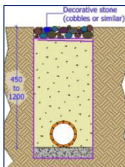
Figure 3.1 - Filter Drain under pavement (left)
