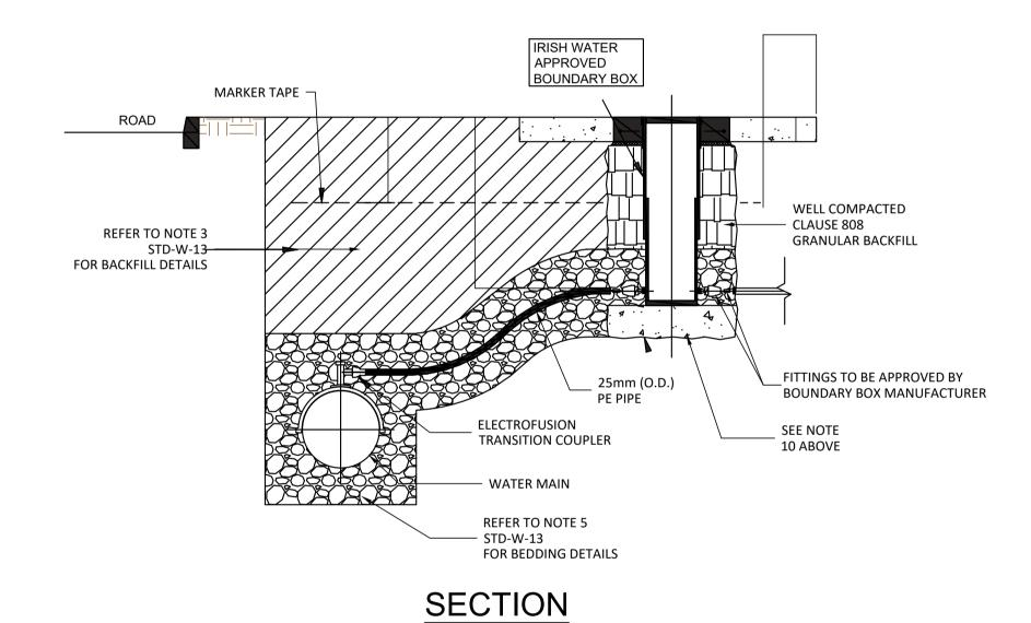
CUSTOMER CONNECTION AND BOUNDARY BOX (25mm OD PIPE)
