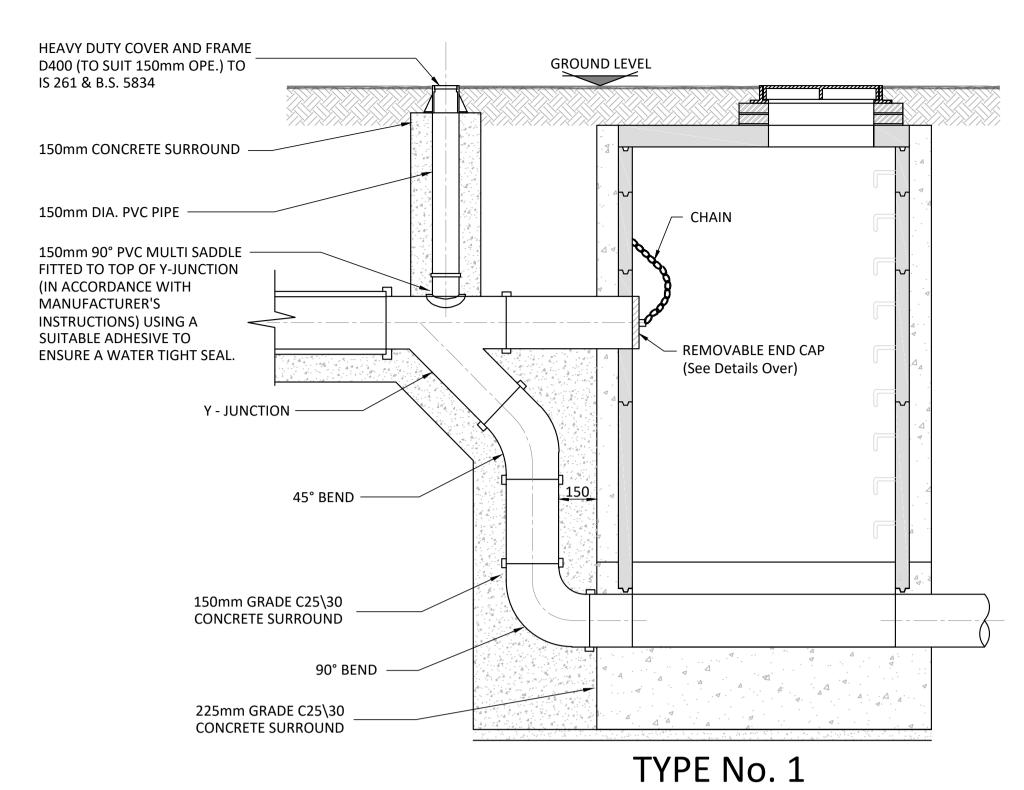
150mm - 450mm DIA. (INCL.) DROP GREATER THAN 1700mm & LESS THAN 2300mm 500mm - 900mm DIA. (INCL.) DROP GREATER THAN 2300mm & LESS THAN 3000mm
